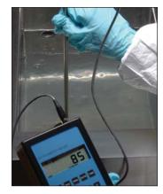
Our digital hand-held meters allow users to map the in-situ energy distribution, establish tank-to-tank uniformity, and identify debonded or failed transducers. This is accomplished through our advance sensor and signal processing design, which captures the cavitation implosion and the driving acoustic signatures.
