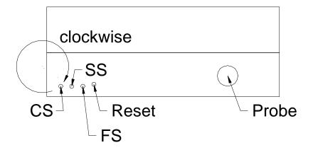
Megasonic cavitation energy meters have two energy calibration screws located on the top of the meter under the receptacle for the Megasonic probe. The locations of the screws are shown on the drawing below. The screws appearing on the right of the meter (with the front side facing towards you) are used to calibrate the energy readings. The screw on the left will be called the **Calibration Screw (CS)** and the screw appearing on the will be called the **Sensitivity Screw (SS)**.
