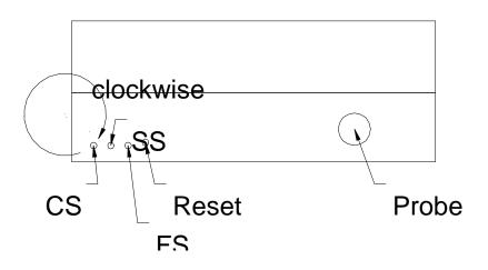
Ultrasonic cavitation energy meters have a **calibration screw (CS)** located on the top of the meter behind the receptacle for the ultrasonic probe. The location of the screw is shown on the drawing on the previous page. The **SS** and **FS** screws are disabled on the pb-500 meter. The procedure to calibrate the energy with this adjustment is as follows:
